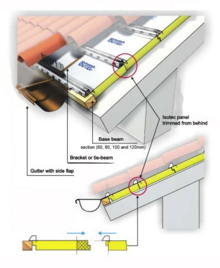
Lay wood beam at edge of eaves (i.e. use a 6x6 for Isotec 6 cm panel and 8-10-12 cm for other thickness). Attach gutter so it overlaps the wood beam. The gutter can also be secured later. Size the eaves panel for width, then lay the first row of Isotec panels at the eaves. Lay the second row of Isotec panels after removing the tooth under the contour so that it adheres to the Isotec panel at the eaves. Continue with more layers as far the ridge.
