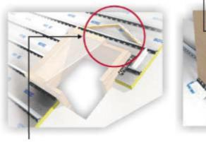
V protection against leaks above the technical structure
