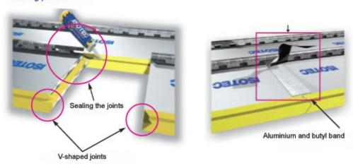
When laying staggered joints, silicone the panels and protect with an aluminium and butyl band.
