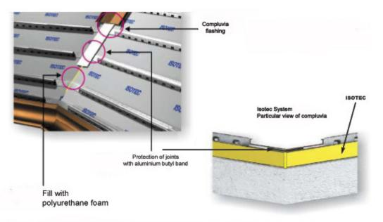
At compluvia and hips, fill any irregular edges with polyurethane foam and protect with aluminium butyl band. Compluvia should also be finished with tin trimming to match the top roofing layer. Incompatible metals should be separated by sheath.
